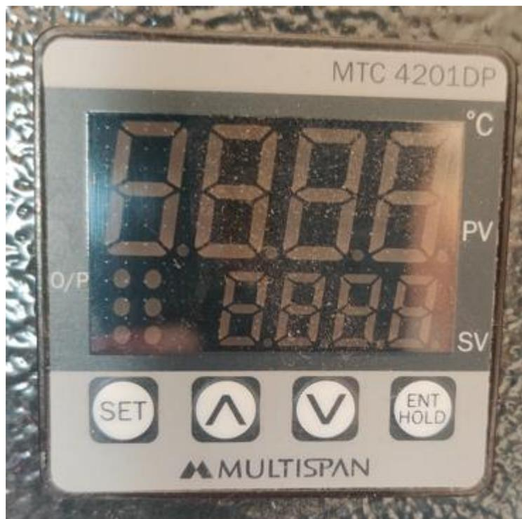
Figure 2: Digital temperature controller
